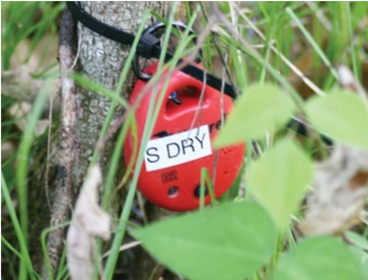
Located at the base of a tree, a Kestrel weather meter records the hourly temperature, dew point, relative humidity, and heat stress index.
